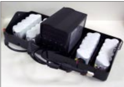
The charger automatically recharges two sets of batteries. It restores 60% capacity in 60 minutes, 90% in 90 minutes, and fully recharges a set in two hours. The tray simplifies staging in large facilities.
